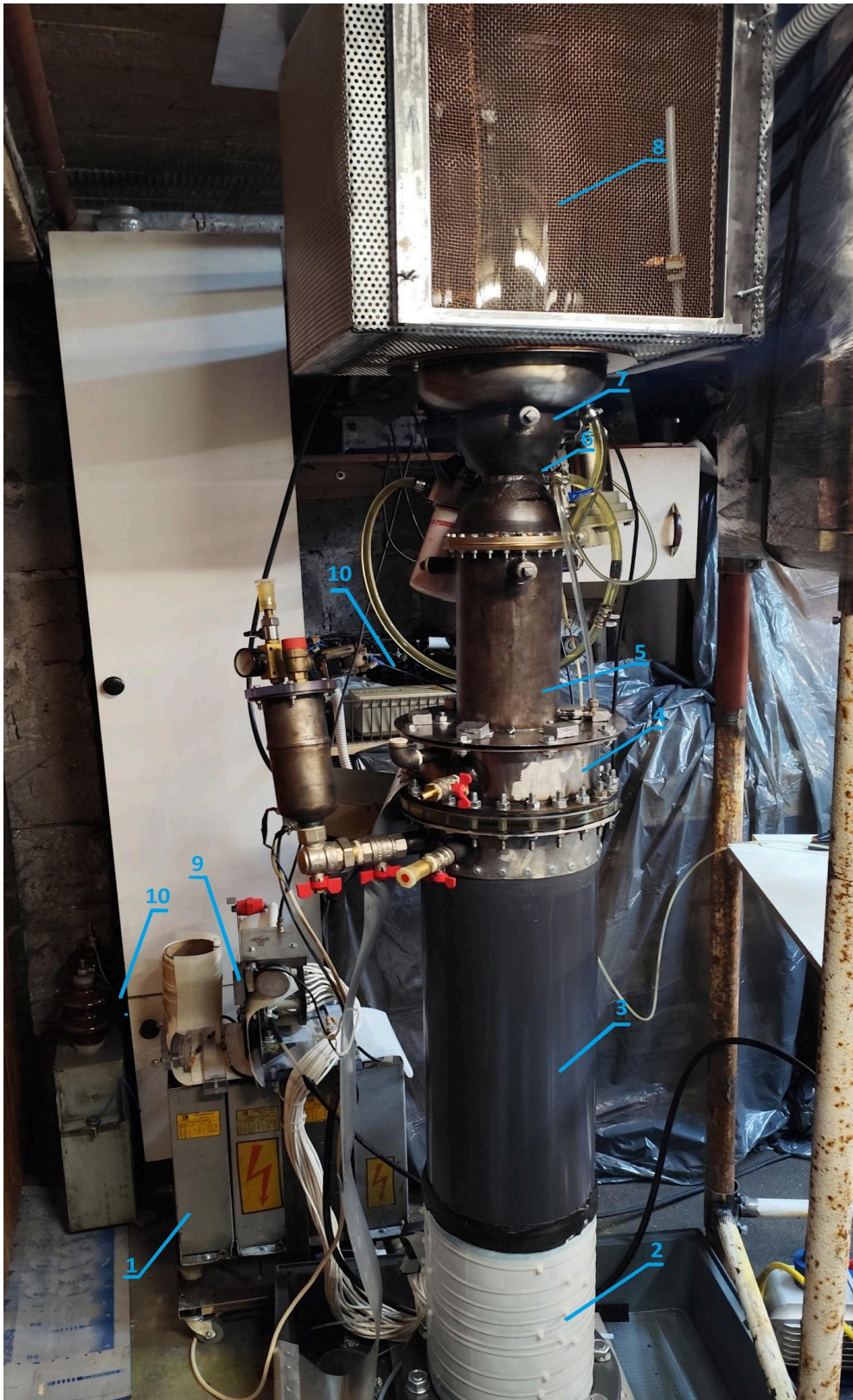
Fig. 2. Photograph of the experimental setup. 1 – main energy storage capacitor bank, 2 – primary winding of Tesla transformer, 3 – mylar-glycerol line, 4 – oil line, 5 – triacetin line, 6 – oil spark gap, 7 – oil line and diode connection, 8 – vacuum chamber and diode in Faraday cage, 9 – trigatron assembly.
