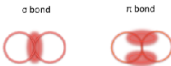
Figure 10.2 Schematic figure of the overlapping of the electron clouds is shown in 2D for \sigma and \pi bonds.
